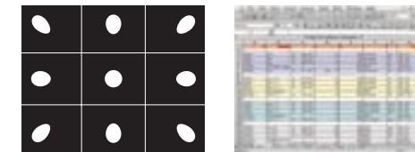
Image without AccuBeam adjustment. Projectors without zone focus capability exhibit softer corner and edge sharpness.
